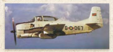
Look Ma, no tail hook! Tail hooks were removed, and cowl strakes were added to allow spin recovery with armaments on combat T-28Cs.
